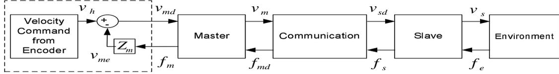
Figure 1. Telerobotic network
